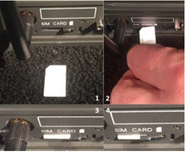
Installing SIM card and engaging the lock
