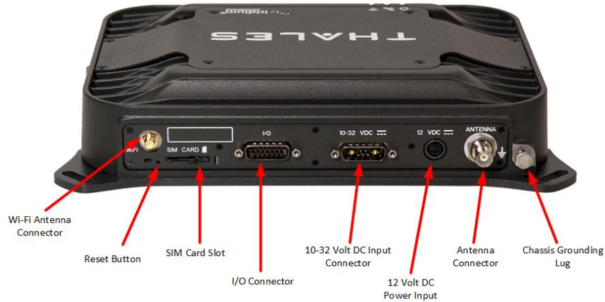
Figure 1-5 Terminal Unit (TU) Back Panel Detail
