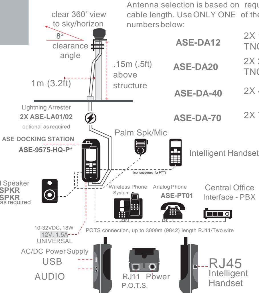
Antenna selection is based on required cable length. Use ONLY ONE of the part numbers below:
