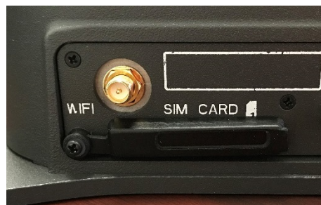
Figure 2-9 Secure the SIM Card Cover
