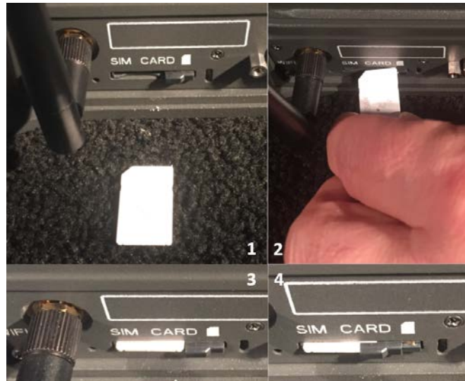
Figure 2-8 Installing SIM Card and Engaging the Lock
