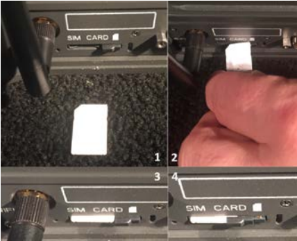
Installing SIM card and engaging the lock
