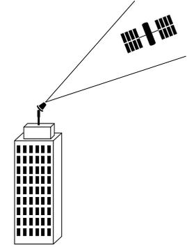
The antenna must be installed without obstruction of other instruments or structures. The antenna must not be positioned within range of radar equipment or other RF interference.
